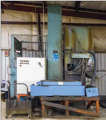
Steimel Chip Reclamation System
