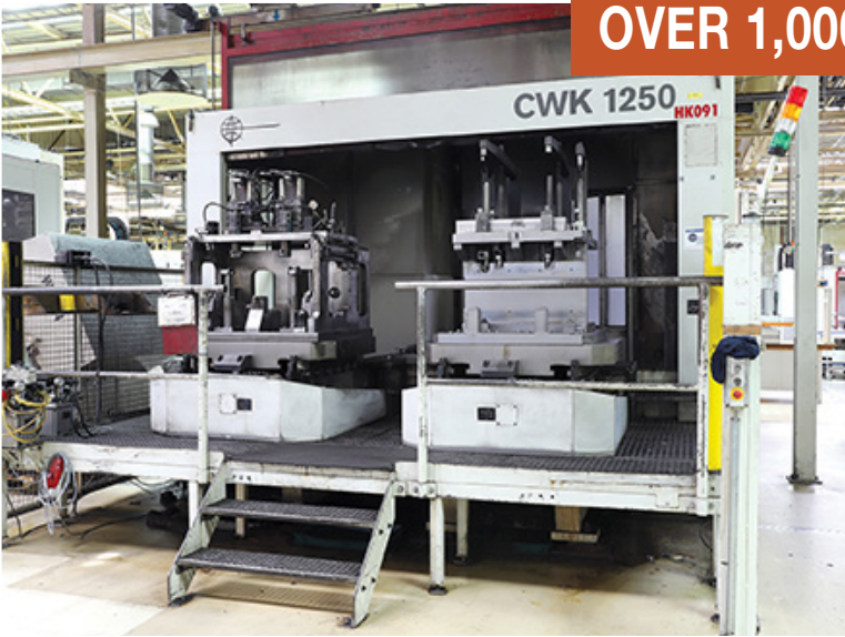
STARRAG-HECKERT CWK 1250 Horizontal Machining Center, for Workpieces up to Diameter 1,800x1,550mm, Spindle 20 - 6,000rpm, HSK-A 100 40kW 1,200Nm
