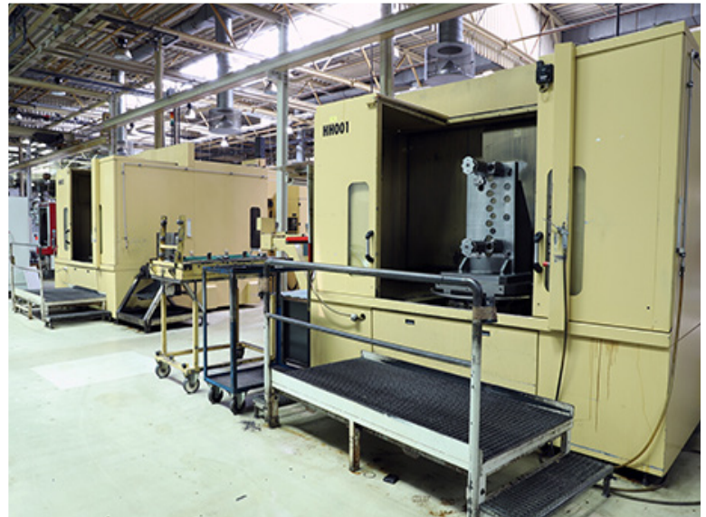
HUELLER-HILLE NBH 230 R Horizontal Machining Center, X/Y/Z 1,200/1,000/1,000mm with B-Axis, Spindle 7,500rpm / HSK-A 100, ATC 80, Feeds 60m/min, Pallet 630x800mm
