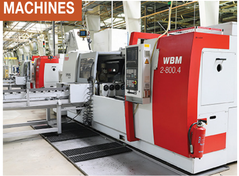
SAMAG WBM 2 - 800.4 CNC 4-Spindle Deep Drilling Machine, Min/Max Diameter 2, 5-18mm, Max Drilling Depth 800mm, Z/W 800mm, 4 Spindles 5, 5/7, 7kW 0-10,000rpm / HSK 80
